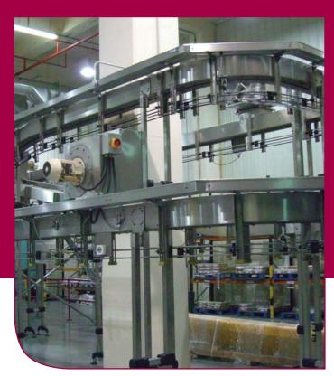
SISMATICO HAVE A UNIQUE NECK GUIDING CONCEPT THAT PROVIDES THE CUSTOMER WITH A 150M JOINT FREE SOLUTION TO ENSURE SMOOTH PRODUCT FLOW. SYSTEMS ARE POWERED BY 3.0KW FAN UNITS POSITIONED AT 10M INTERVALS. VARIOUS GRADES OF FILTRATION CAN BE PROVIDED UP TO 3 STAGE HEPA.
